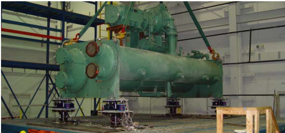
Figure 6. Shake table testing of HVAC equipment on acoustic isolation/restraint systems.
