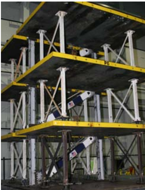
Figure 8. Shake table testing of a 3-story steel frame incorporating Buckling Restraint Braces (BRB) and floor isolation system.
