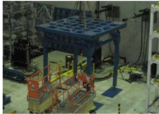
Figure 7. Nonstructural Component Simulator (NCS) at the University at Buffalo, a) bi-axial configuration, b) uni-axial configuration
